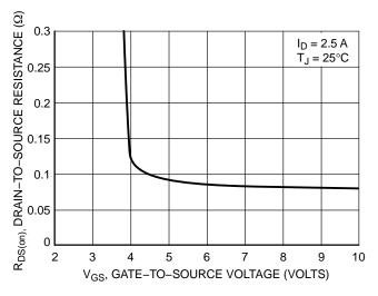
Figure 3. On-Resistance vs. Gate-to-Source Voltage
