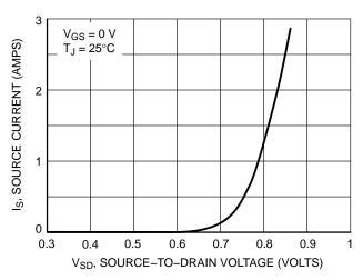
Figure 10. Diode Forward Voltage vs. Current
