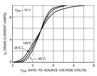
Figure 2. Transfer Characteristics
