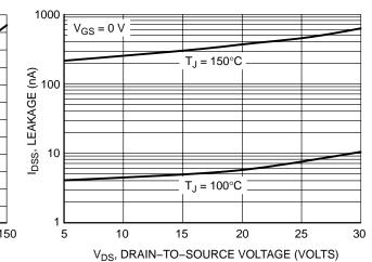
Figure 6. Drain-to-Source Leakage Current vs. Voltage
