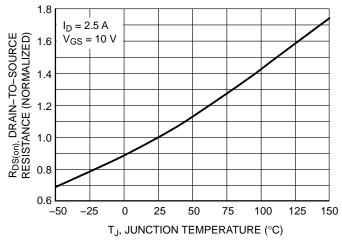
Figure 5. On–Resistance Variation with Temperature
